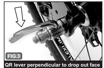
QR lever perpendicular to drop out face
